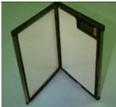
An X-ray cassette used in radiography.
