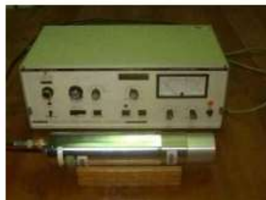
A single channel analyser with a crystal-PMT assembly.
