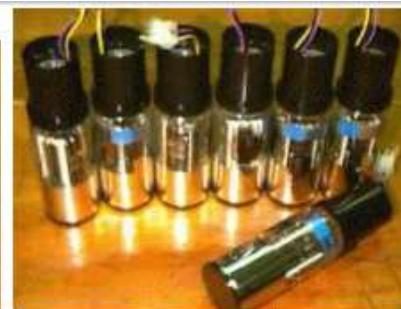
A number of identical photomultiplier tubes from a Gamma Camera.
